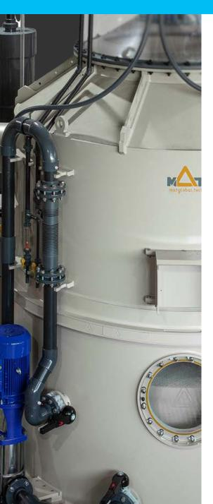
MAT-KULING spent over 12 months testing different venturi injectors on skimmer bodies while feeding tank water with special venturi pumps to obtain the needed pressure and achieve high levels of air infusion into the water cyclone within the skimmer body. After many trials and FEA studies our fresh water protein skimming is now achieving equal, if not better to salt water viscous results.
